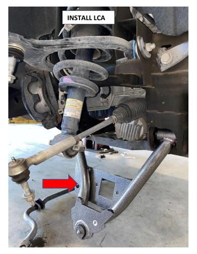
13. Raise lower arm upward and bolt up lower strut hardware. TORQUE TO 45 FT-LBS.
