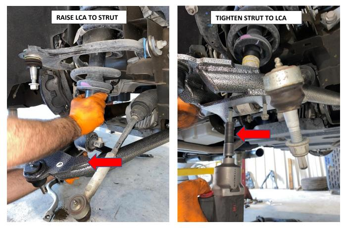
14. **APPLIES TO ONLY 1418LCA**. NOTE: 1418 stamped steel arms has a machined sleeve on lower ball joint that must be inserted in spindle.
