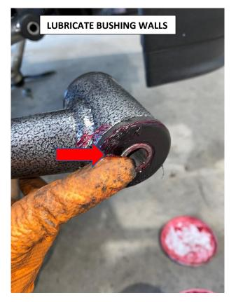
12. Install IHC LCA. DO NOT TIGHTEN!
