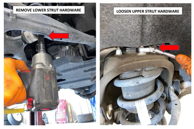
8. Remove lower control hardware and remove OEM LCA.
