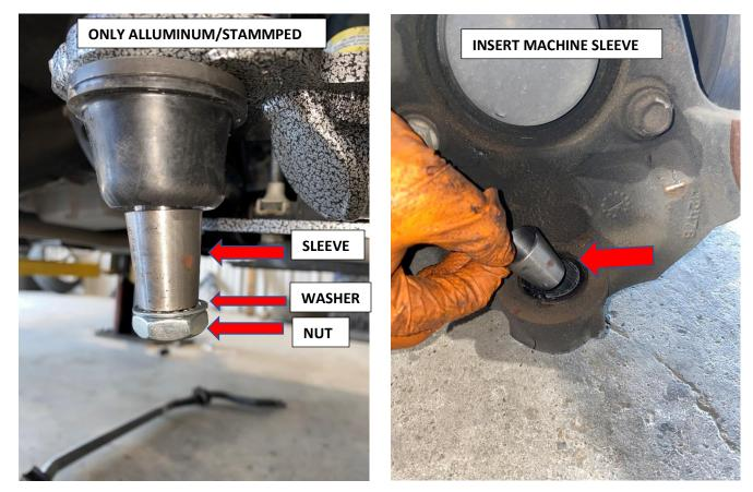
Install OEM spindle to lower control arms. 0713 CAST install castle nut and cotter pin. TORQUE 110 FT-LBS
