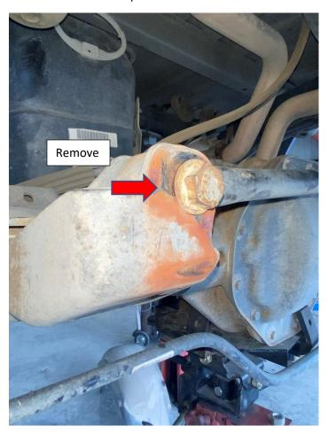
8. Insert suitable tool under differential to prevent diff from pivoting forward. Refer to pic
