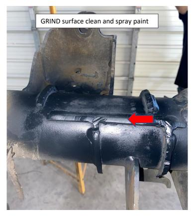
15. Cut off rear bump stops and spray paint to prevent rusting. Refer to pic
