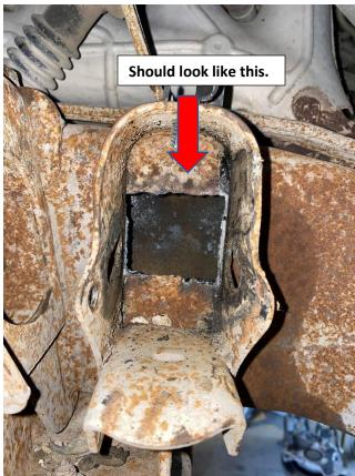
11. Lubricate upper and lower controls frame pocket.
