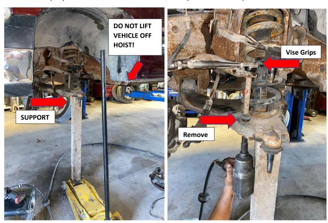
7. Remove lower and upper shock hardware. NOTE: MAKE SURE LCA STILL HAS PRESSURE UPWARD.
