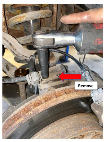
4. Remove the brake caliper and properly secure. NOTE: DO NOT OVEREXTEND BRAKE HOSE
