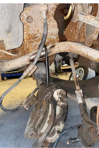
5. Loosen the upper/lower ball joint nut. Strike the ball joint boss on the knuckle with a dead blow hammer to dislodge the taper.
