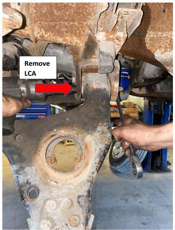
10. ONLY necessary PASSENGER SIDE FRONT SIDE. NOTE: This will allow control arm to have more adjustment.
