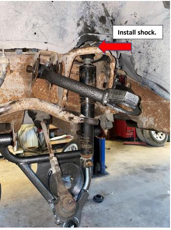
15. Install OEM spring and mount shock to lower control arm. Carefully raise lower control arm until lower shock can mount to LCA. TORQUE TO 18FT-LBS.
