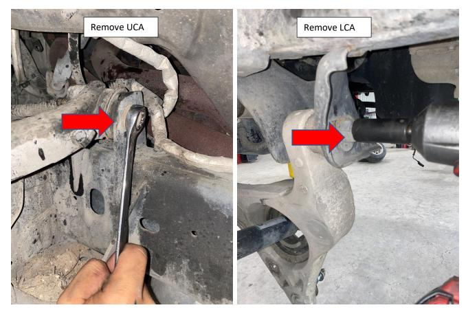
12. Front suspension should be dissembled. Refer to pic
