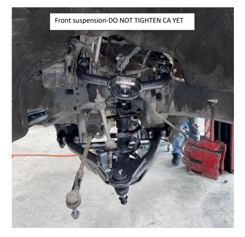
27. Remove OEM sway bar link refer to pic.
