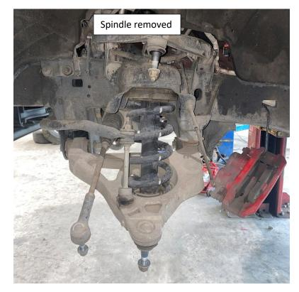
7. Remove lower sway bar link from LCA. Refer to pic
