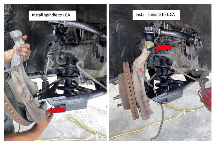
32. Make sure upper control arm has 2 5/8" gold washer installed before castle nut ensure proper installation. The lower ball joint cotter pin will need to be opened to install. Refer to pic
