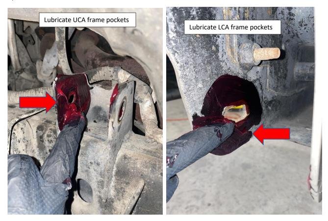
17. Install ZERK fitting on upper and lower control arms. Refer to pic
