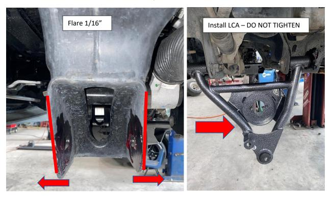
23. Install OEM shock to LCA and with floor jack support IHC LCA. Install OEM spring onto LCA. Refer to pic
