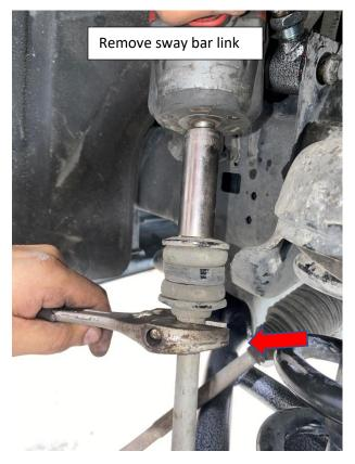
28. You will need to trim sway bar link thread on the side that attached to LCA to allow easier installation of OEM hardware. Refer to pic
