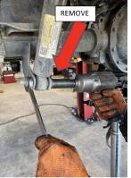
48. Remove the brake line bracket. It's located on the inside of the frame rail on the driver's side of the vehicle. Remove the two bolts that mount the bracket and retain hardware. Refer to the picture on the right.
