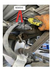
50. Remove the ABS sensor harness bracket from the top of the rear differential. Retain the factory hardware will be re-used.
