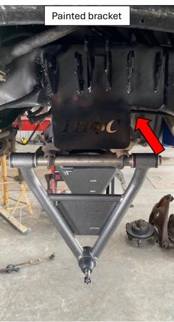
**NOTE:** Driver side UCA is bent differently to allow more room for the power steering box when installed.
