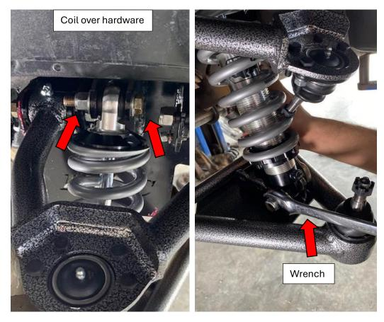
22. Install spindle, lightly torque down upper and lower ball joints with castle nut and install cotter pin.
