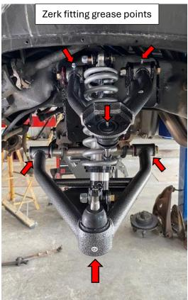
PLEASE READ IMPORTANT NOTE: IHC front coil over is already assembled. Thread lower collar down to apply ANTI-SIEZE on threads. Failure to do so will result in damage to coil over and VOID warranty.
