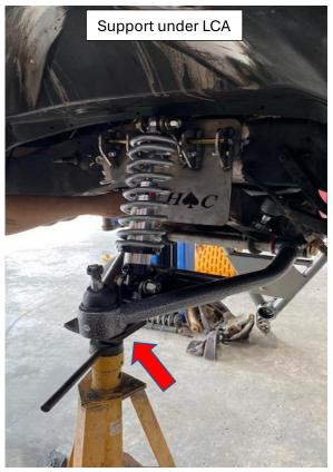
**HOW TO CENTER:** With the LCA and coil over mocked up you will place the upper IHC bracket with coil over as square as possible, tack IHC plate, then measure from the edge of the plate facing towards rear of the truck to the center of the body mount. That measurement will be your center reference for the other side as well.
