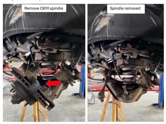
**8.** Apply upward pressure to LCA before removing shocks and sway bar links, then slightly remove pressure from LCA and remove springs/shocks. **NOTE: Spring may still be under load. Please be cautious when removing.**
