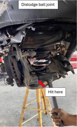
7. Remove spindle assembly.
