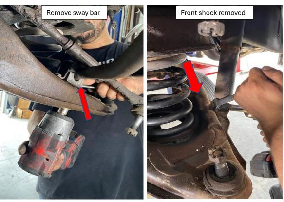
9. Remove front coil spring from the LCA. **NOTE: Spring may still be under load. Please be cautious when removing.**
