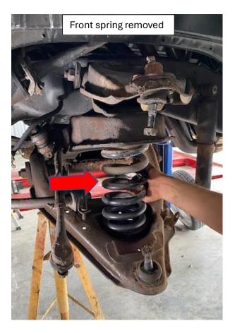
10. Remove upper and lower control arms. NOTE: In some cases, LCA hardware may need to be cut off.
