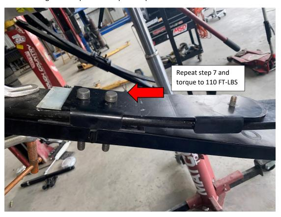
10. Raise leaf pack and re-install flip kit. Torque u bolts 110 FT-LBS
