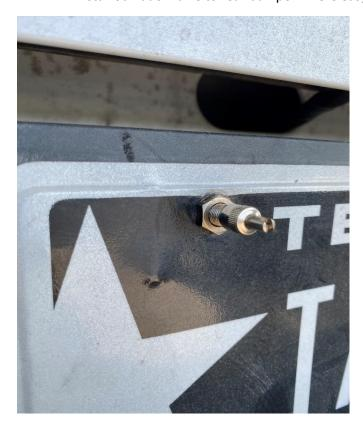
18. Air up air bags 50 psi and let sit for 30 min. Recheck air pressure of maintain 50psi your installation is complete. If lost air pressure with soapy water check all fitting and airlines. Repair as necessary.
