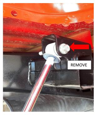
4. Remove rear u bolts along with flip kit Top plate, and bottom plate.
