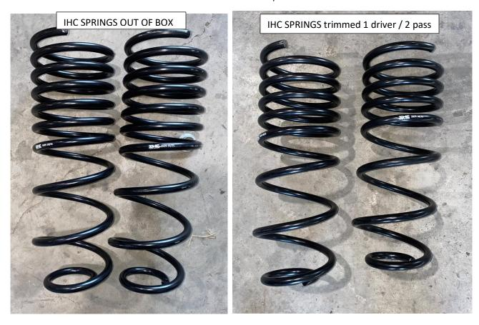
27. Install OEM isolator on top of IHC springs and install IHC Springs. NOTE: LOWER IHC SPRINGS NEED TO BE CLOCKED AS PICTURE. FAILURE TO DO SO WILL RESULT PUSING SPRING TOO FAR BACK. Refer to pic
