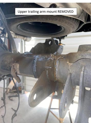
14. After cutting grind surfaces down to give clean look and spray paint to prevent surface rusting. Refer to pic
