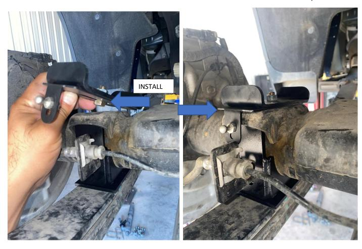
9. Once vehicle is on the ground install sensor rod. Refer to pic
