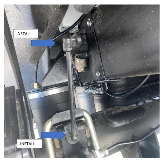
10. Install IHC shock extenders. Torque shock hardware to 80ft-lbs Refer to pic
