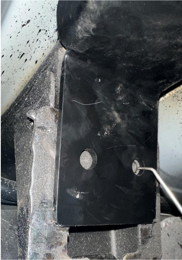
80. Drill holes with 3/8" drill bit. Refer to pic.
