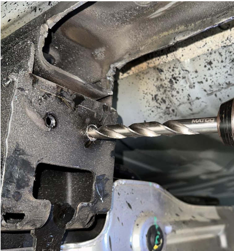
80. Drill holes with 3/8" drill bit. Refer to pic.
