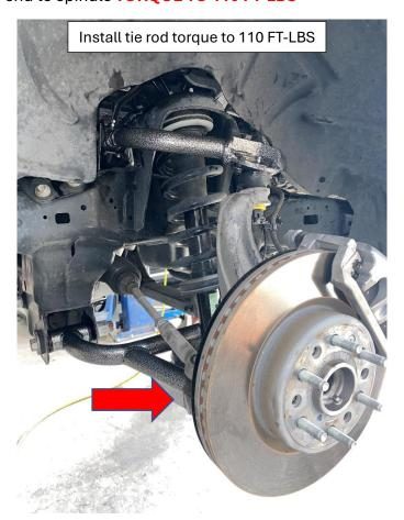
**37.** Lubricate all ball joints and control arm bushing. Refer to pics below.
