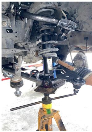
28. Insert lower strut bolt and tighten down firmly. Torque upper strut hardware to 45 ft lbs.
