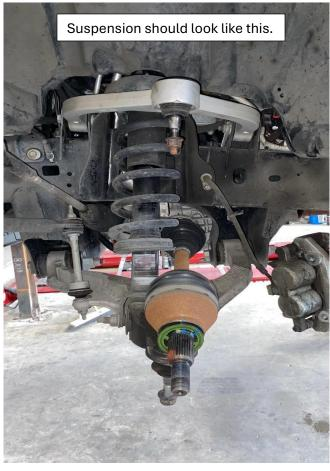
8. Remove sway bar link from LCA.
