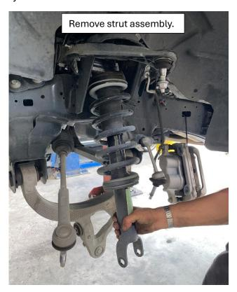
**12.** Remove lower control arm hardware and lower control arms.
