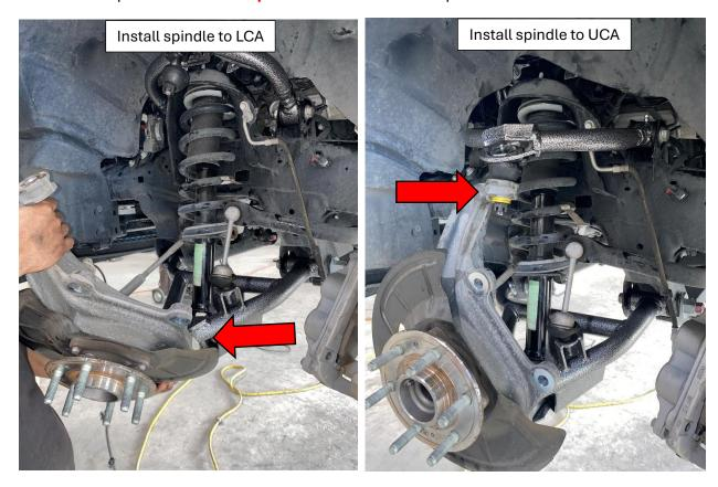
**30.** Install and tighten UCA. Install 5/8 gold washers prior to installing castle nut **torque to 65ft lbs** and install cotter pin. Refer to pic
