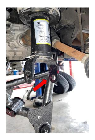
27. Raise IHC lower control arm up. In some cases you will need to apply upwards pressure to align holes to install hardware. If on post lift, place a sturdy mount under LCA and safely lower vehicle to align holes. If installing on the floor, use a floor jack to apply upward pressure to align holes. NOTE: When raising LCA, make sure it does not lift from hoist/jackstands.
