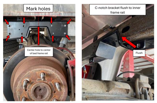
9. Drill the holes using a <sup>1</sup>/<sub>2</sub>" drill bit. **ONLY DRILL OUTER SECTION OF FRAME.** Refer to pic
