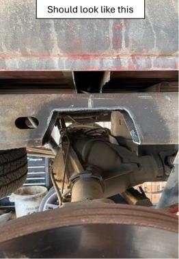
8. With the c-notch installed against the outside face of the frame rail, use a paint marker or center punch to mark all the holes outside the frame. Refer to pics.
