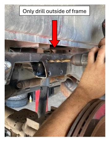
10. After drilling, use the c-notch stud hardware to check for fitment and clearance.
